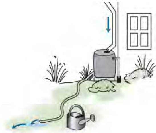
Examples of rainwater harvesting (Source: United States Environmental Protection Agency)
