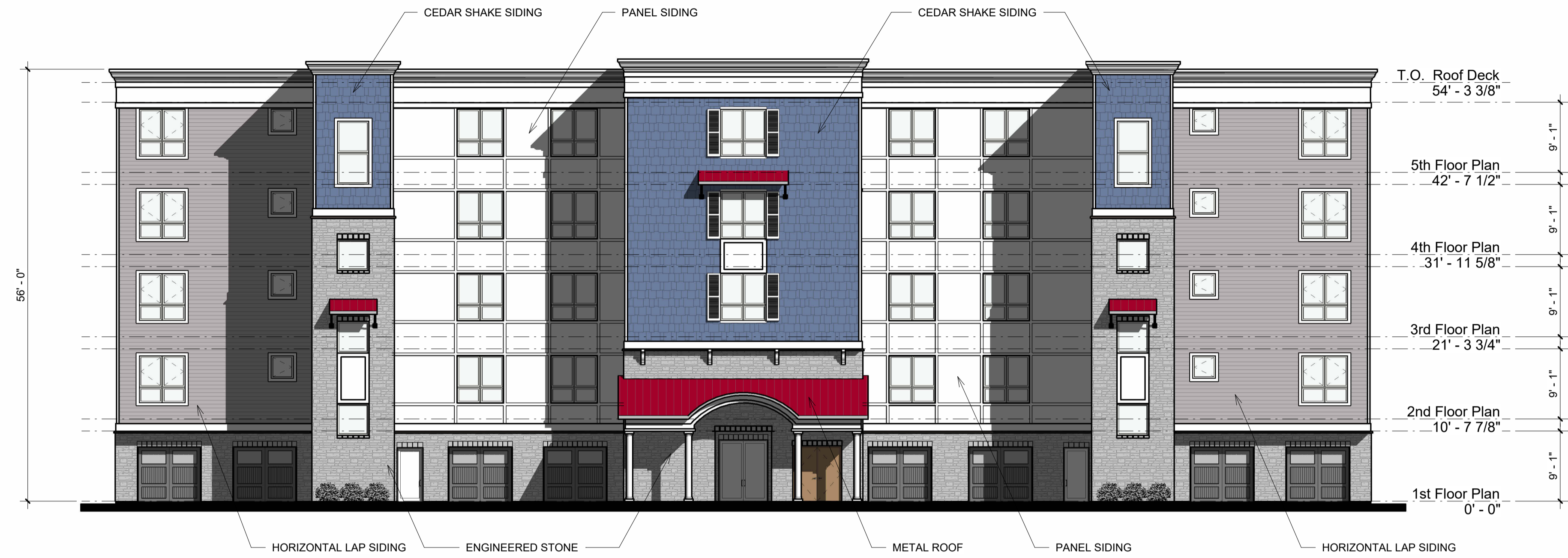
Bldg. 1 & 3 - Front Elevation Scale: 3/32" = 1'-0"
