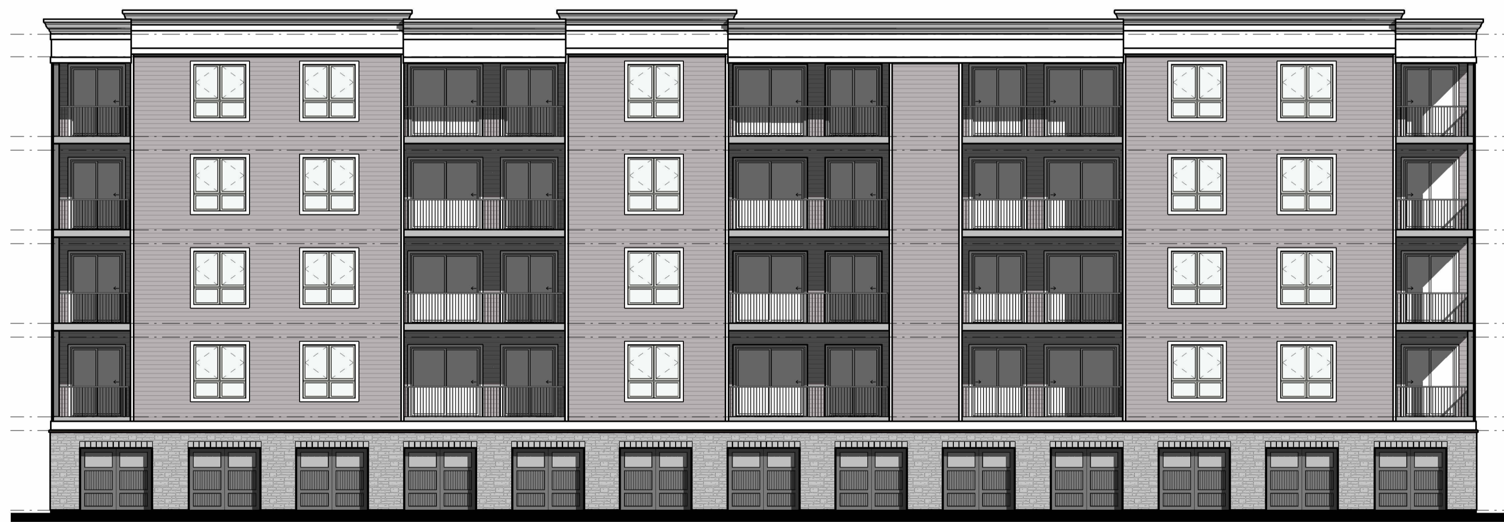
Bldg. 1 & 3 - Rear Elevation Scale: 3/32" = 1'-0"
