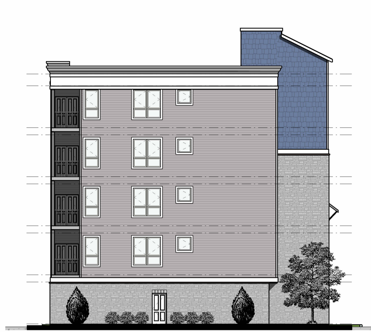
Bldg. 2 - Left Elevation Scale: 3/32" = 1'-0"
